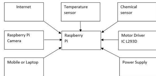
**Fig.1. General Block Diagram**
