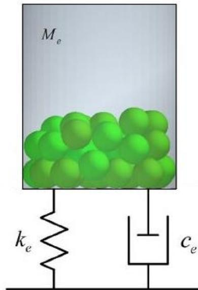
Figure 2 Single degree of freedom particle damper [7]
