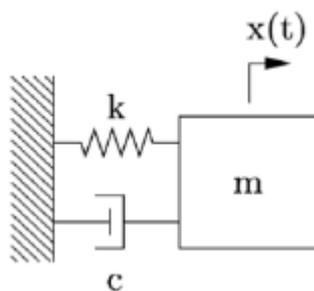
Figure 1 Elements of vibratory system [2]
