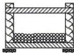
Figure 3 Schematic of particle damper
