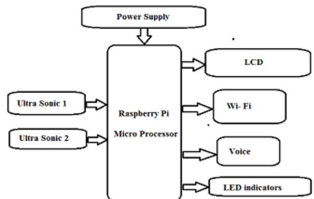
The reason for using two radar sensors is to recognize the direction from left to right, or from right to left, of the moving human. That is, through two thin electronic layers, a human passing by radars is detected, and counting is performed in both directions. For this purpose, the two radar sensors are designed to be spaced by a certain distance  $d$ .
