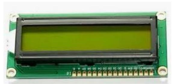
Fig 4: 16\*2 LCD Display.
