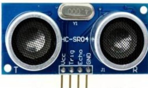
Fig 3: Ultrasonic sensor (HC-SR04)
