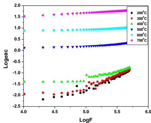
**Fig. 8** Variation of ac conductivity with frequency for different temperature of Sr<sub>2</sub>FeNiO<sub>6</sub>.
