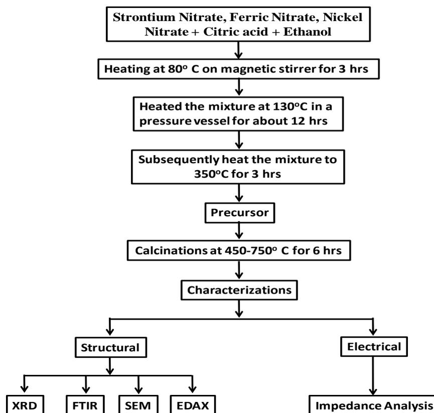
**Fig. 1** Flow chart for the preparation of  $\text{Sr}_2\text{FeNiO}_6$  double perovskite nanocomposites.
