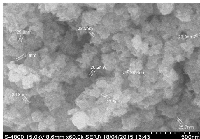
**Fig. 4** SEM image of  $\text{Sr}_2\text{FeNiO}_6$  DP nanocomposites.
