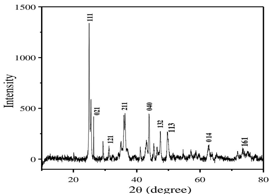
**Fig. 2** X-ray diffraction pattern of the synthesized  $\text{Sr}_2\text{FeNiO}_6$  calcined at  $650^\circ\text{C}$ .
