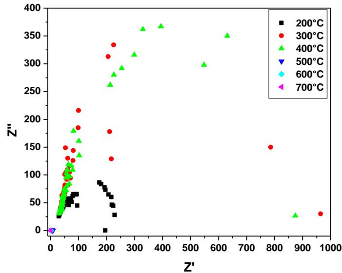
**Fig. 7** Complex impedance spectra of the nanocrystalline Sr<sub>2</sub>FeNiO<sub>6</sub> at different temperatures.
