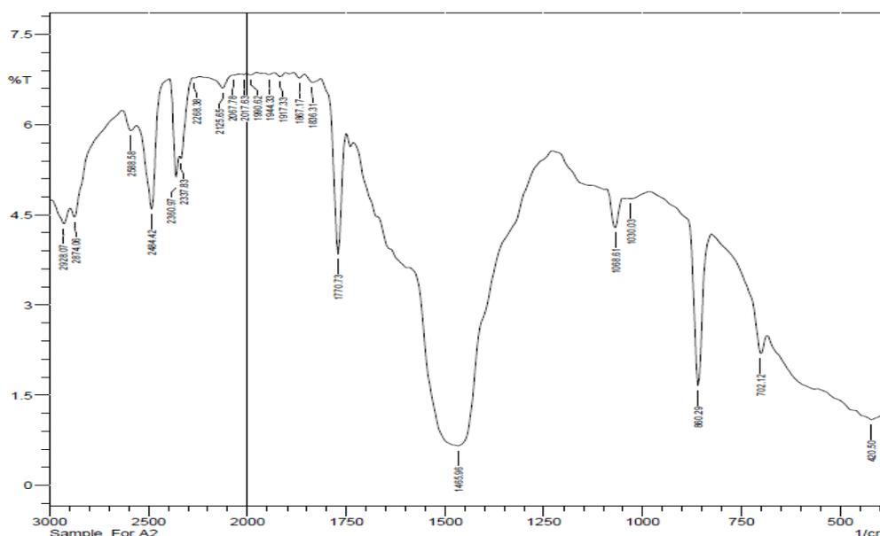
**Fig. 3** The FTIR spectrum of  $\text{Sr}_2\text{FeNiO}_6$  nanocomposites calcined at  $650^\circ\text{C}$
