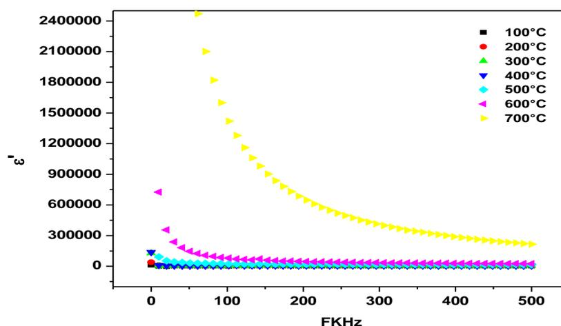
**Fig. 6** Dielectric constant of the nanocrystalline Sr<sub>2</sub>FeNiO<sub>6</sub> at different temperatures.
