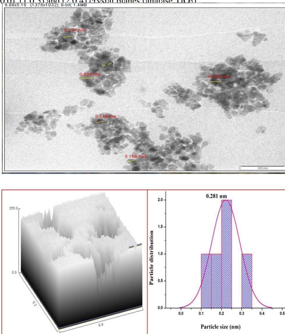
**Fig.2.** HR-TEM analysis of  $\text{Bi}_2\text{O}_3$ - $\text{TiO}_2$  nanocomposite material (a) TEM Image (b) Surface plot and (c) particle size in selected area highlighted fig (a)
