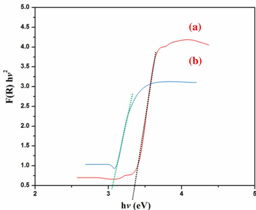
Fig 5. UV-Vis DRS analysis  $TiO_2$  and (b)  $Bi_2O_3-TiO_2$  nanocomposite material
