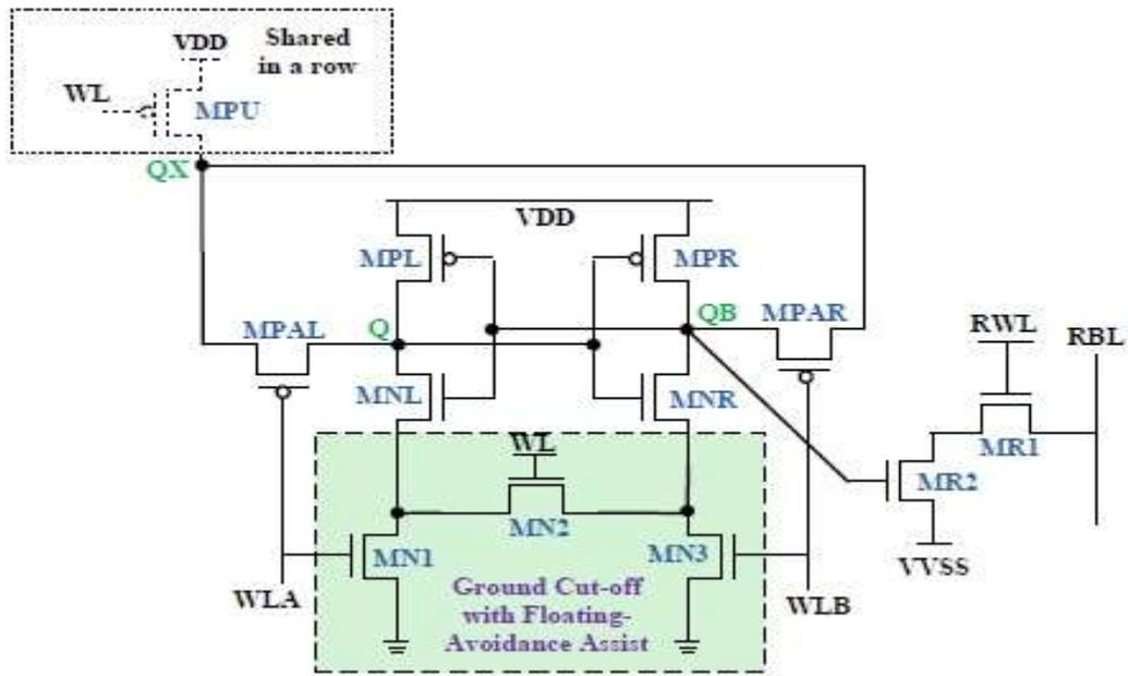
Fig 2 Proposed 11T-2 cell Schematics
