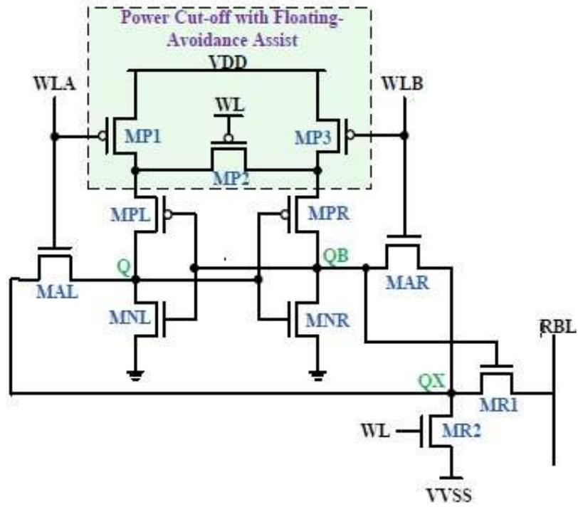
Fig 1 Proposed 11T-1 cell Schematic
