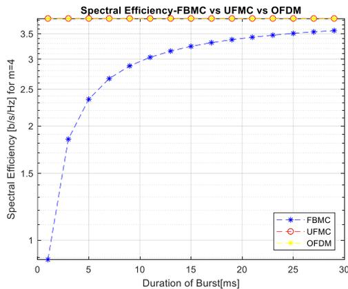
**Fig 5.3. Spectral Efficiency-FBMC vs UFMC vs OFDM**
