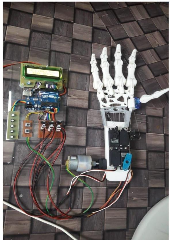
Fig. 3. Prosthetic robotic hand system
