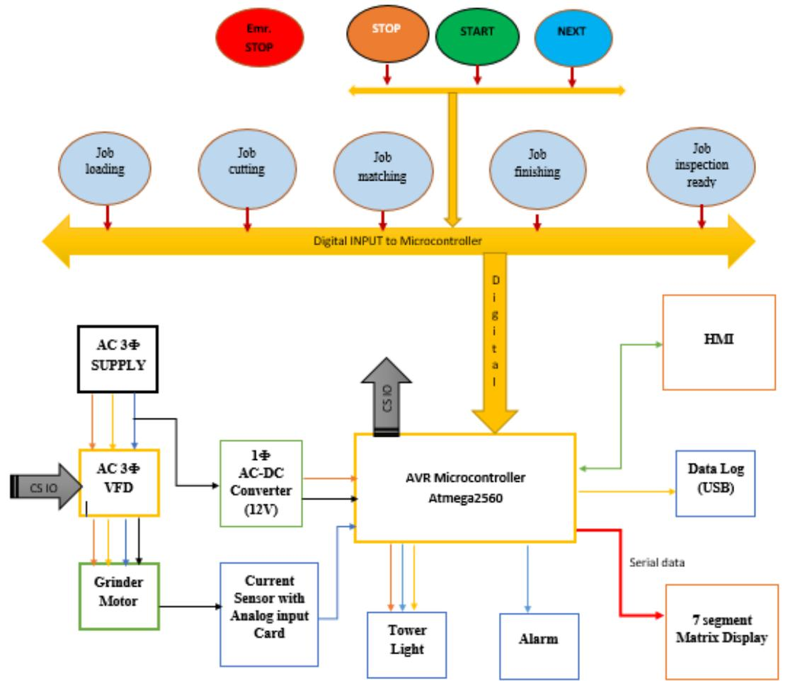
Fig. 1 Block diagram of proposed solution
