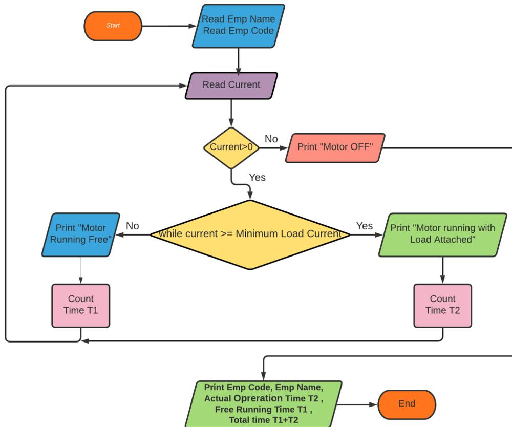
Fig. 2 Flow diagram of proposed solution
