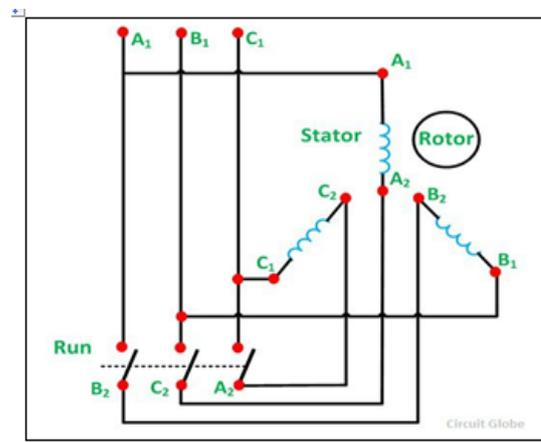
Star delta starter is used to reduce the starting current drawn by the motor. Start the motor in STAR and then, when the motor has gained sufficient speed, change its connections to DELTA to allow the motor to run at its full speed and torque from then on. The motor starts as star connected, ie, voltage reduced by root(3), current reduced by root(3) and power reduced by 3. After the motor starts, it is switched to delta connection and runs normally.
